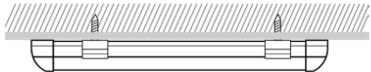
1. Gently press the tube into the metal clips until it is secured properly.
